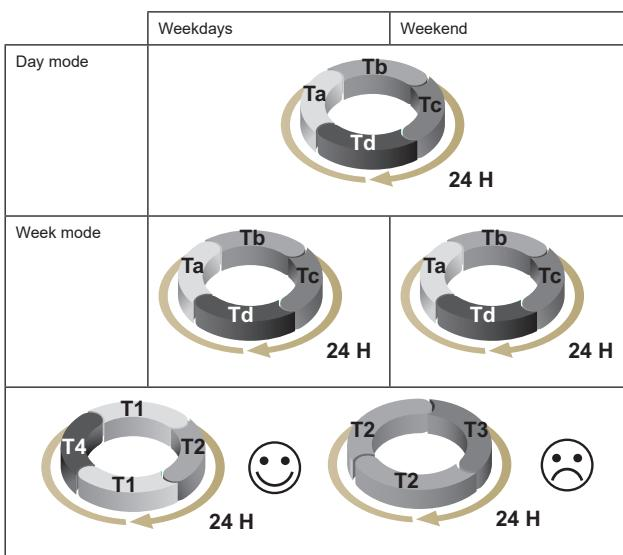
**en** A scheduler supports a maximum 4 time segments (Ta, Tb, Tc and Td) for a maximum 4 tariffs (T1, T2, T3 and T4). You can assign Ta, Tb, Tc or Td to any tariff provided that any adjacent time segment has a different tariff.
